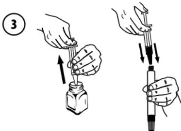
Reference chart below for mixing guide. Use syringe to add recommended amount of Testors 1148 thinner into brush end of marker barrel. Then, use syringe to add paint.
