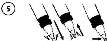
Invert and depress tip several times on a hard surface until thoroughly wet.
